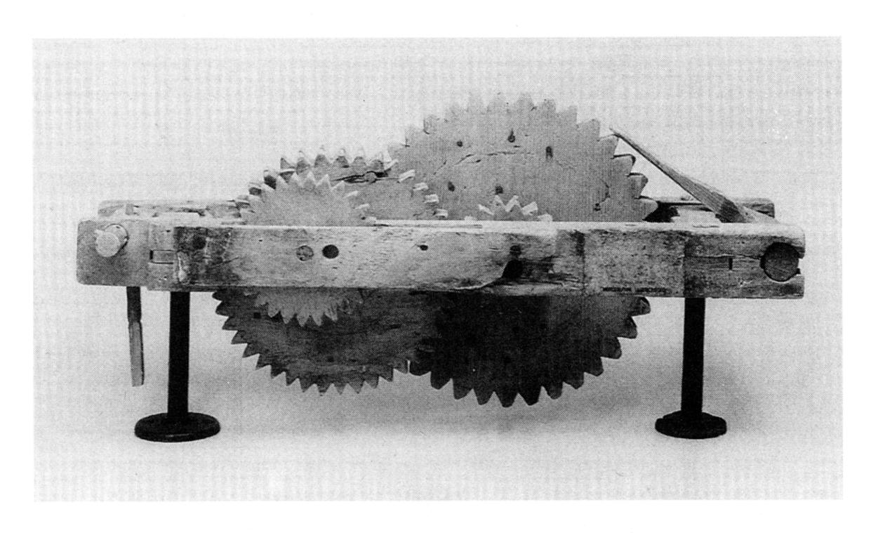
Fig. 1. Thomas Lowe's odometer. For over fifty years, many people believed that this odometer was the first ever invented and that it was designed by Orson Pratt for use by the first company of Mormon pioneers.
