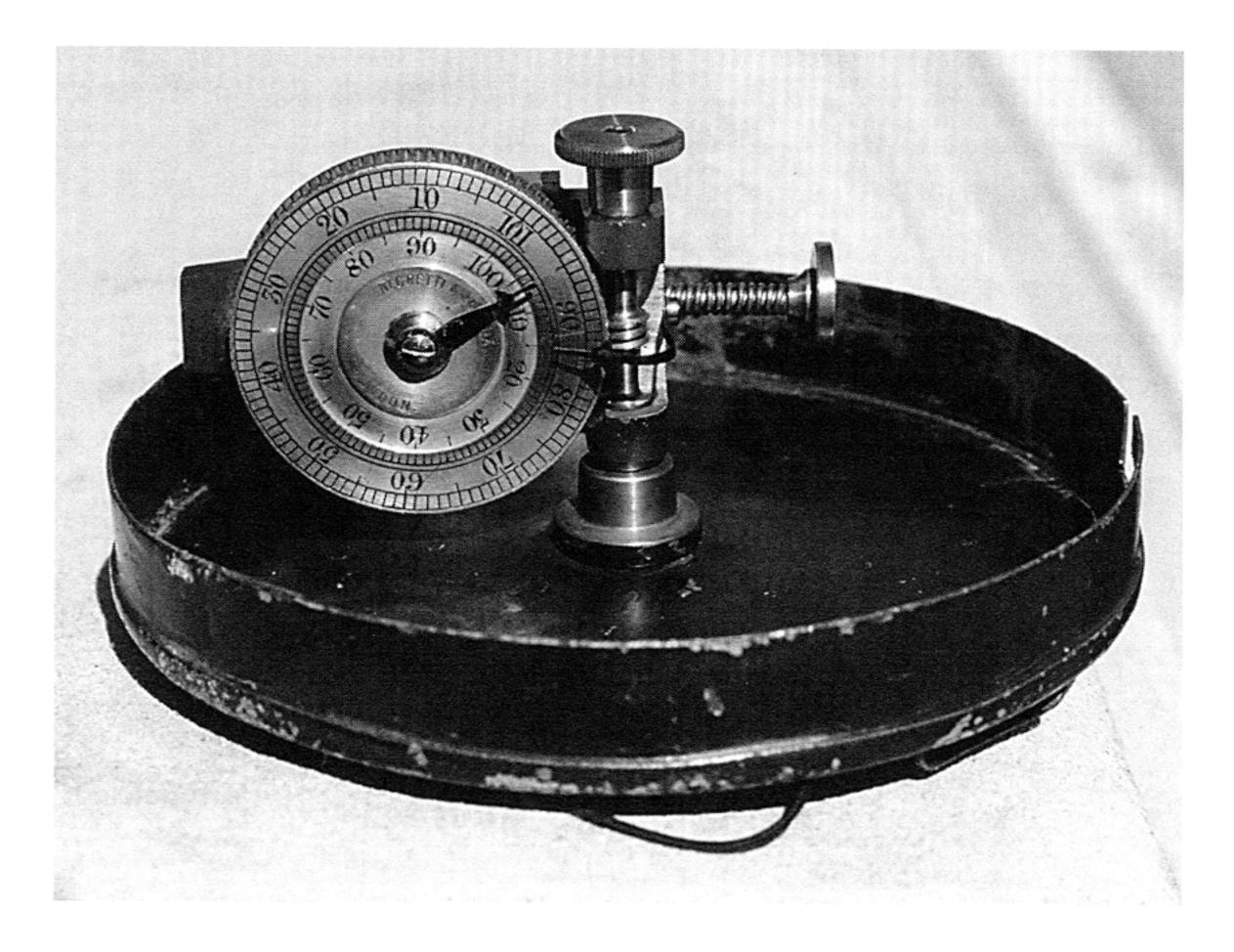
**Fig. 3**. English viometer, c. 1850. Distance-measuring devices such as this were available at the time the pioneers crossed the plains.
