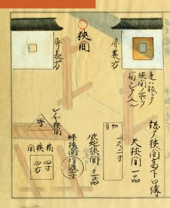
Varying designs for weaponry openings in walls.
